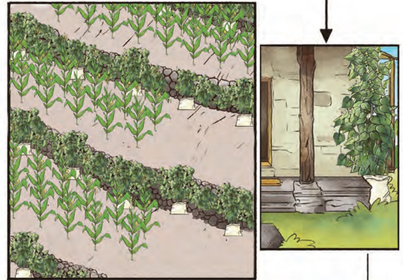
4. Place bags at bottom of terrace wall
