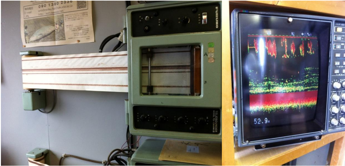
Figure 3.3. Data display devices for conventional equipment. (Left): Thermal paper printing device. (Right): CRT display of fish intensity. Source: Yasui, 2014.
