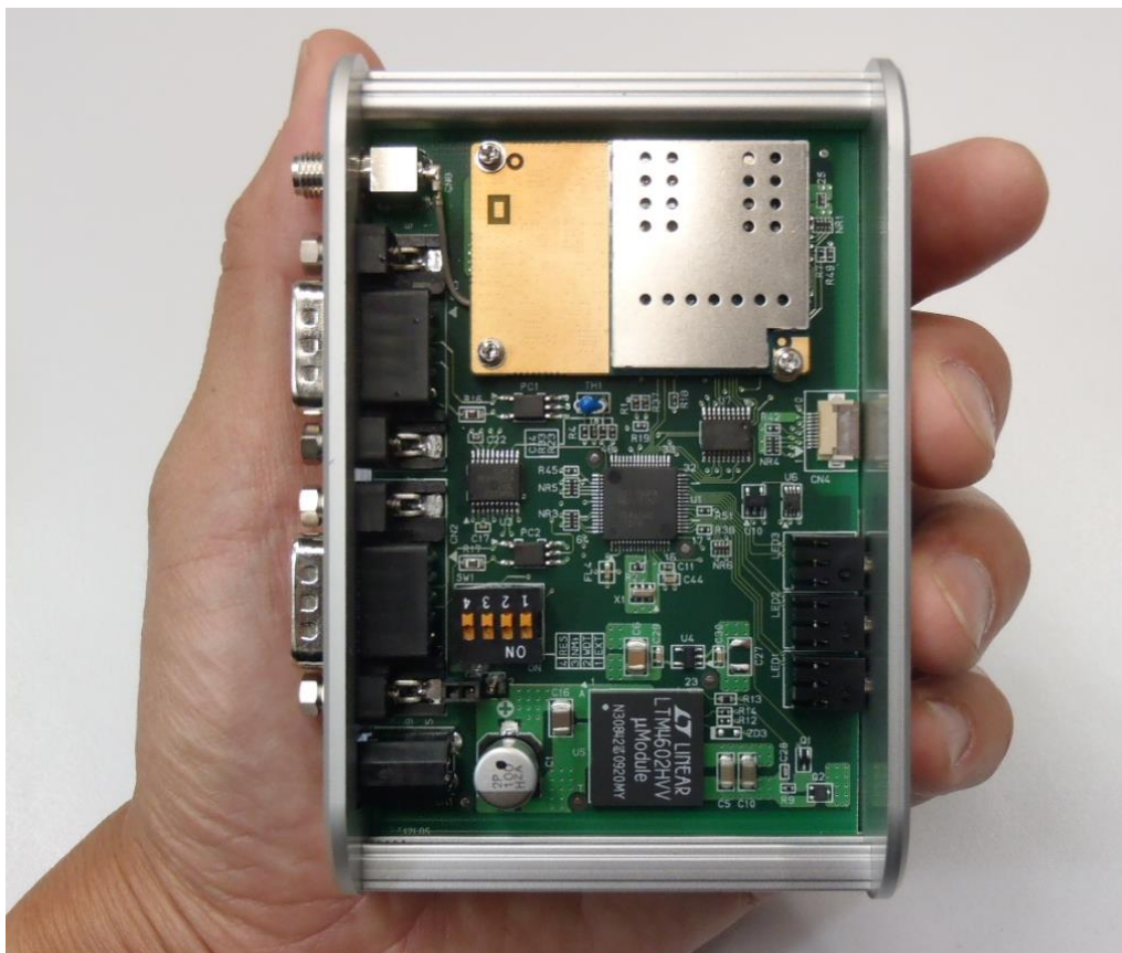
Figure 2.3. Photograph of a microCube unit used in the vessels to collect and transmit GPS data in real time. Source: Wada, 2013.
