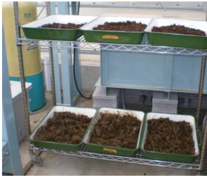
Photo. 6-1 Situation of air drying experiment
