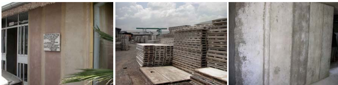
fig 58 – Agrostone production facility and use in social housing. (Pictures Tjerk Reijenga)
