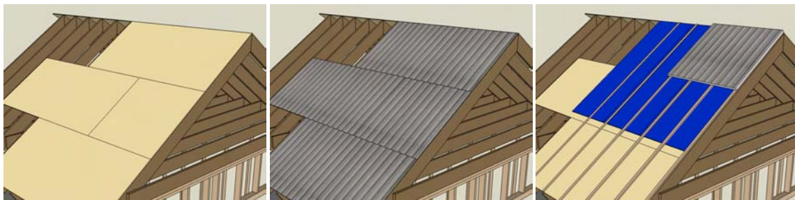
Fig 19 - Plybamboo roof, corrugated iron roof or plybamboo roof with protective (damp-open) sheet and corrugated iron roofing.
