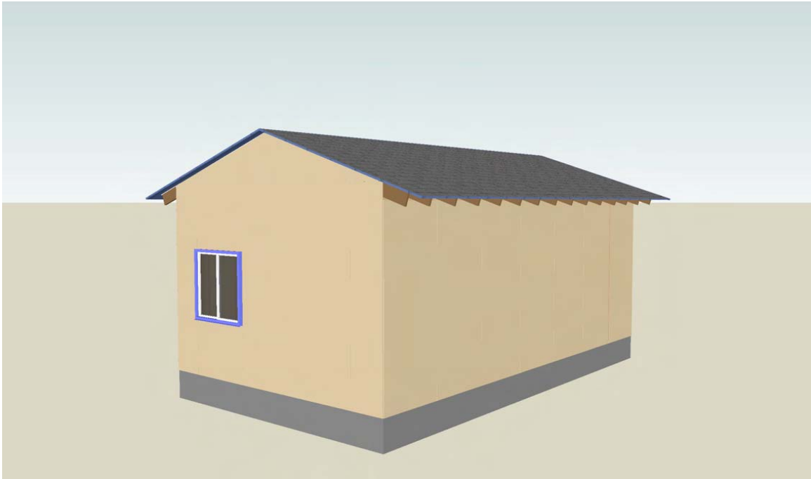
40 m 2 unit - North-east view. Low angle asphalt roof.
