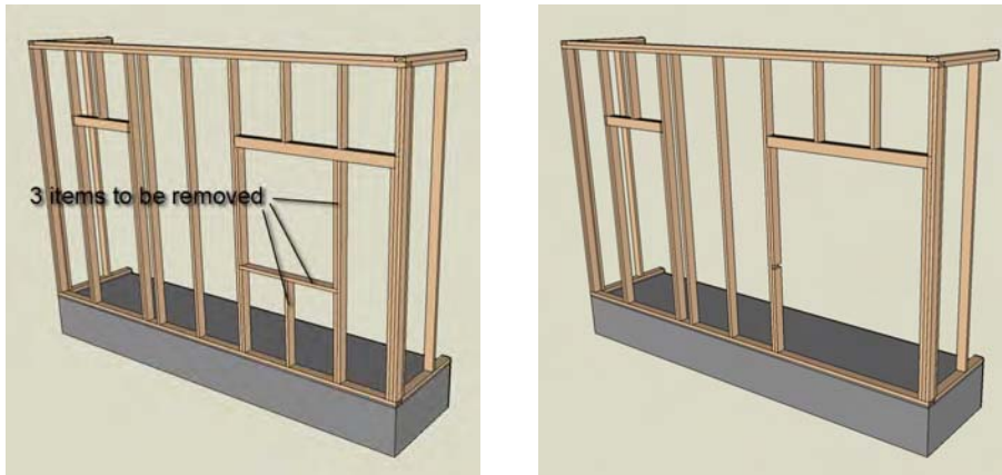
Fig 12. Detail of the wall of the 40 m 2 house and the changes that has to be made for future extension to the 60 m 2 house.
