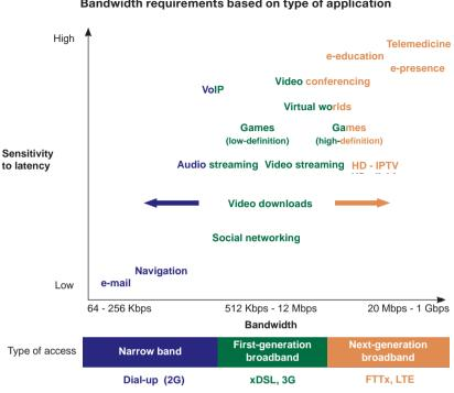
Figure I.2 Bandwidth requirements based on type of application
