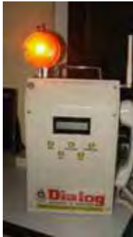
Figure 9 Remote Alarm Device
