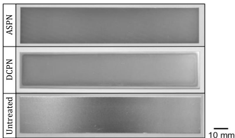
Fig. 6.3 Appearance of untreated and nitrided SUS304.
