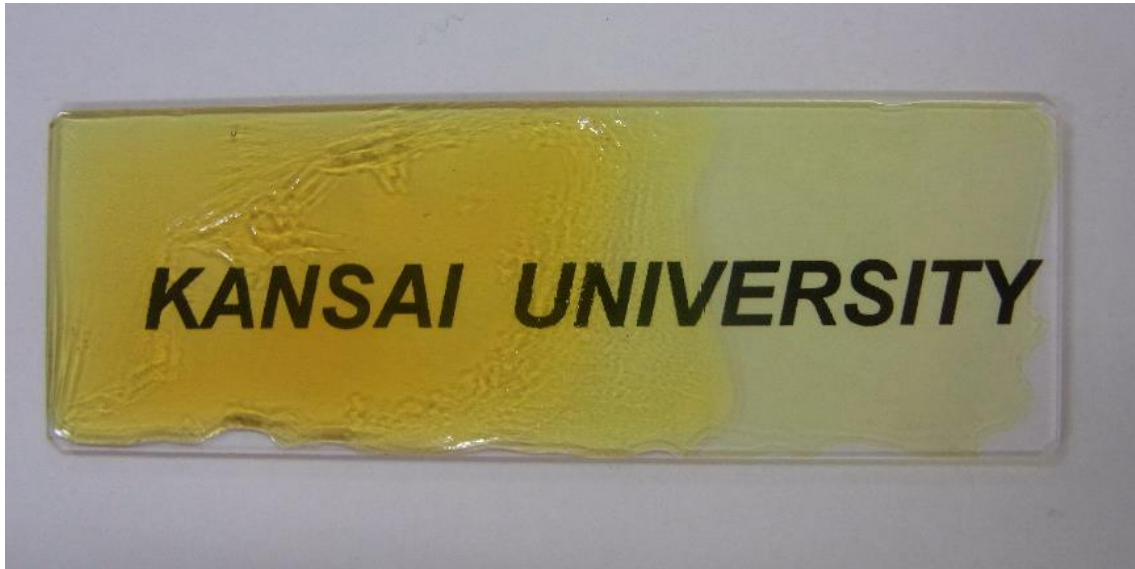
Figure 4.2 Appearance of the 120°C-dried sample prepared on a soda-lime glass substrate. The sample was prepared by dropping the concentrated solution on the substrate.
