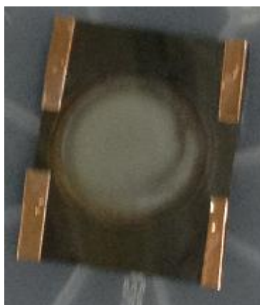
Fig. 5.7 Photo of CuZn/CuSn thin films using the device of the substrate at the bottom of the electrolyte
