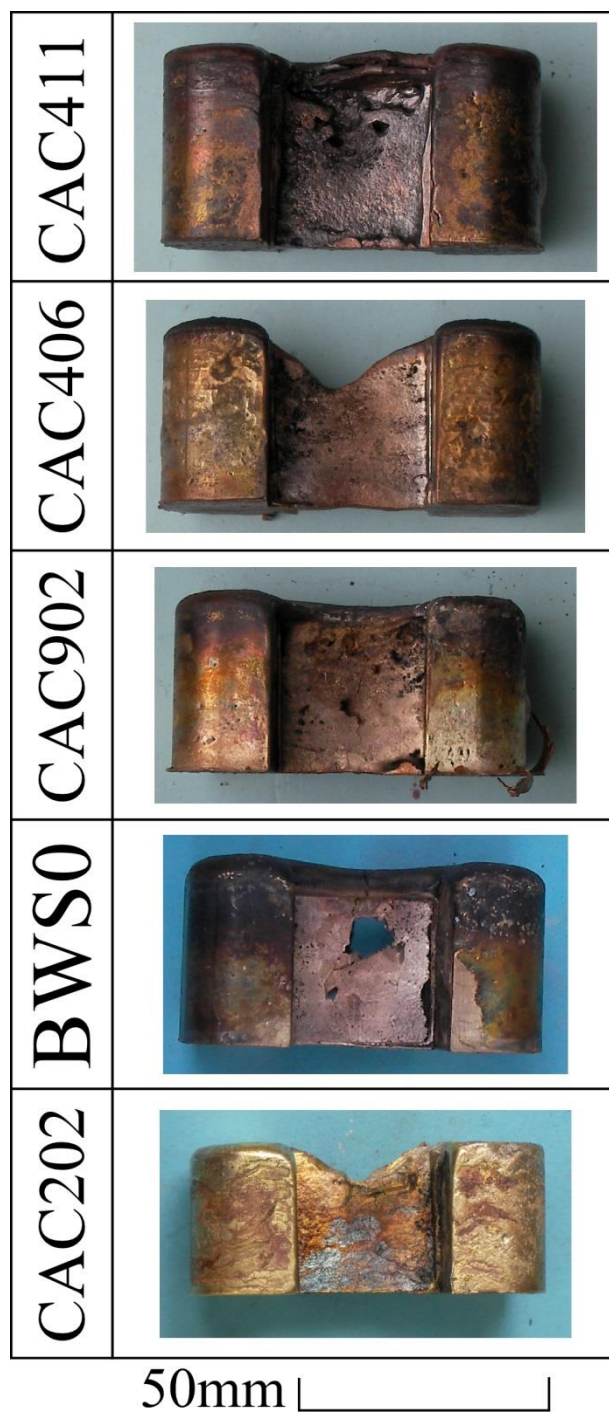
Fig. 4-16 Appearances of various bronze castings in permanent mold for solidification cracking test (Length: 30mm).
