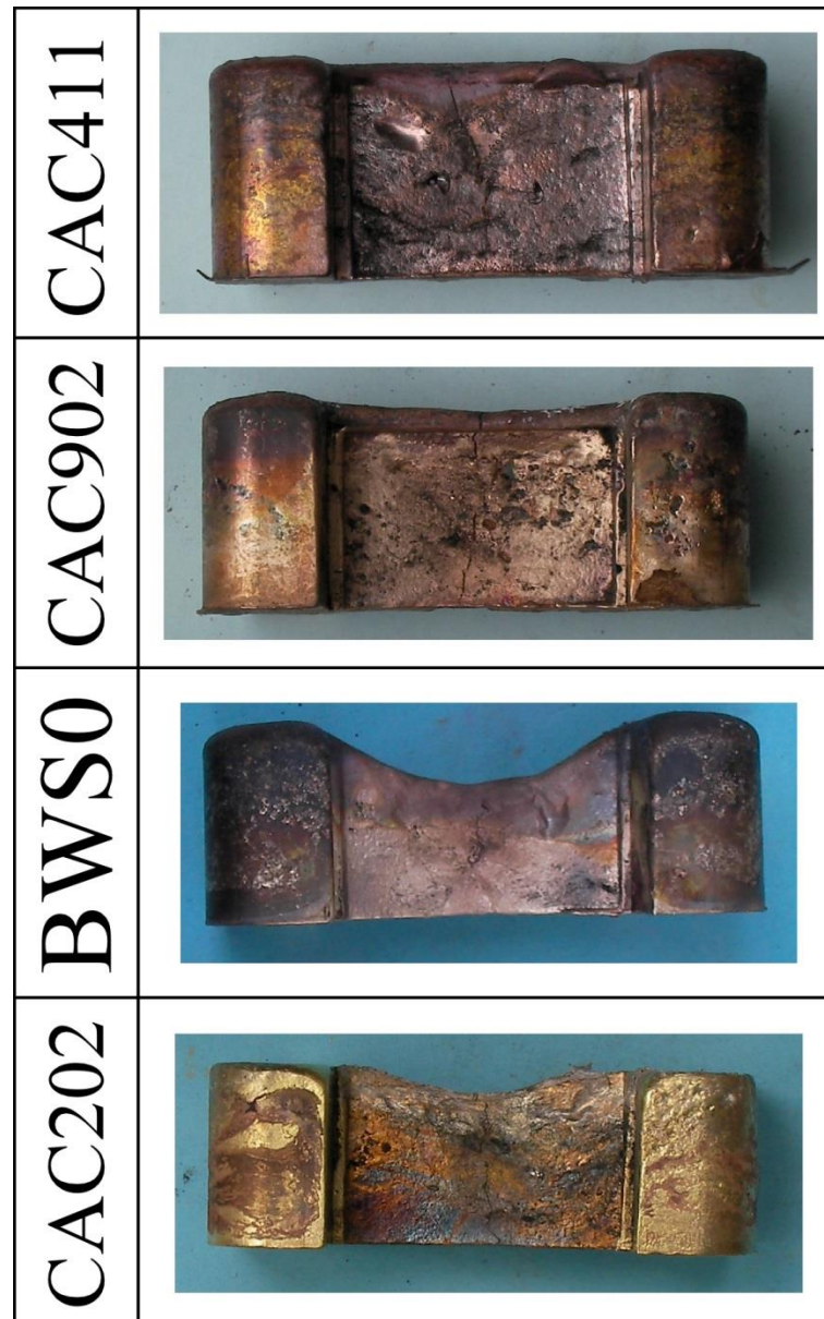
Fig. 4-15 Appearances of various bronze castings in permanent mold for solidification cracking test (Length: 50mm).
