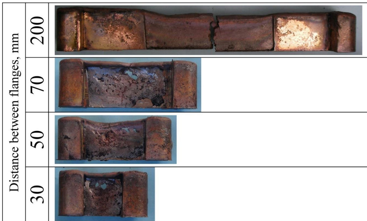
Fig. 5-12 Appearances of BWS42 alloy castings in permanent mold for solidification cracking test.
