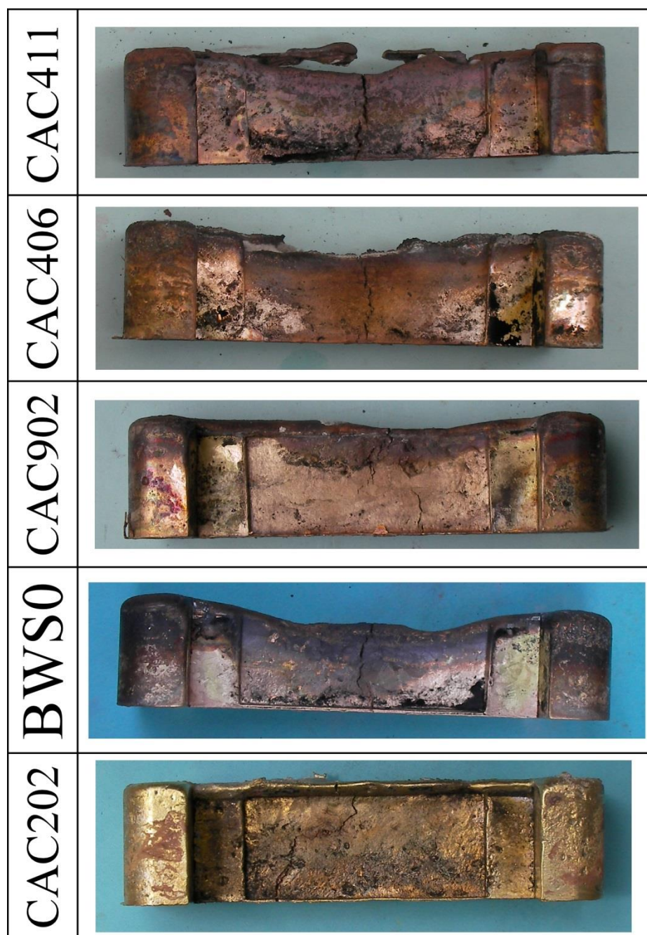
Fig. 4-13 Appearances of various bronze castings in permanent mold for solidification cracking test (Length: 100mm).
