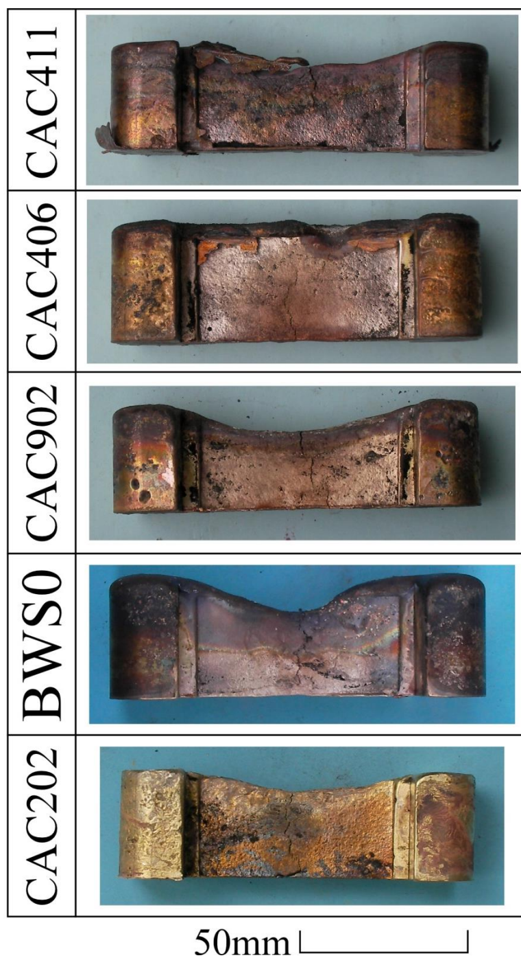
Fig. 4-14 Appearances of various bronze castings in permanent mold for solidification cracking test (Length: 70mm).
