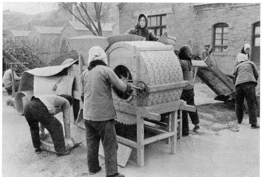
Hand operated sorghum thresher in action at Tachai: a model for increasing productivity.
