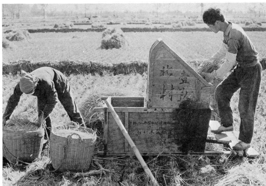
The pedal thresher: it can fill a basket with rice in five minutes.
