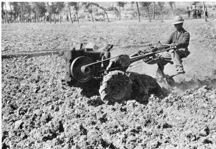
The 10 h.p. “walking tractor” — key to China’s agricultural mechanization program.
