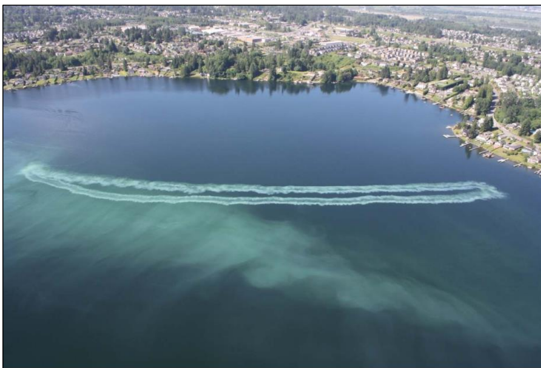
Figure 5-5. Alum treatment in Lake Stevens, Washington
