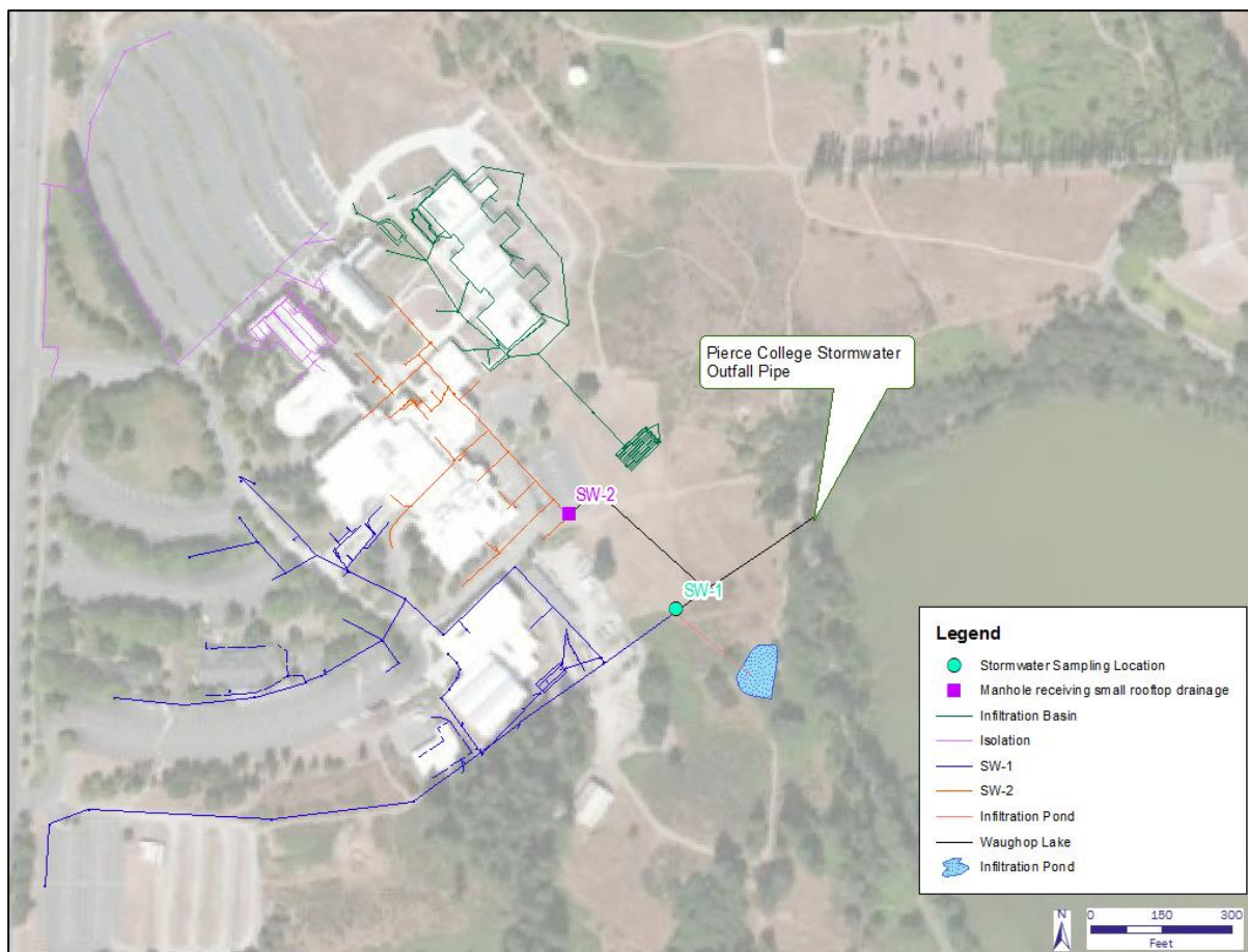
Figure 2-12. Stormwater drainage outfall at Pierce College
