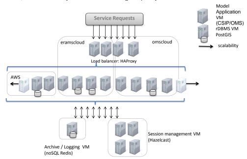
Figure 1. CSIP Physical Architecture.
