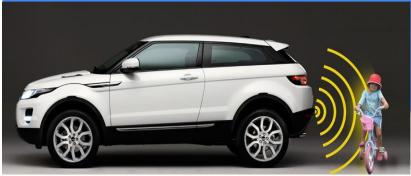
Parking sensors detect objects behind the car and beep to alert the driver
