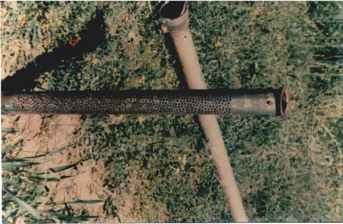
Fig. 5.3: Making the screen lip by Inserting a 2.5 inch metal pipe with a lip inside the original pipe and Fixing it with a bolt and screw.
