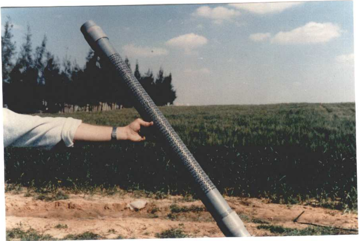
Fig. 5.8 The Modified PVC. Screen
