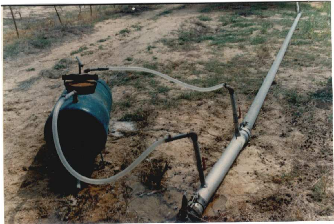
Fig. 5.13 The Modified Fertilizer Tank Used with the Hand-Move Sprinkler System
