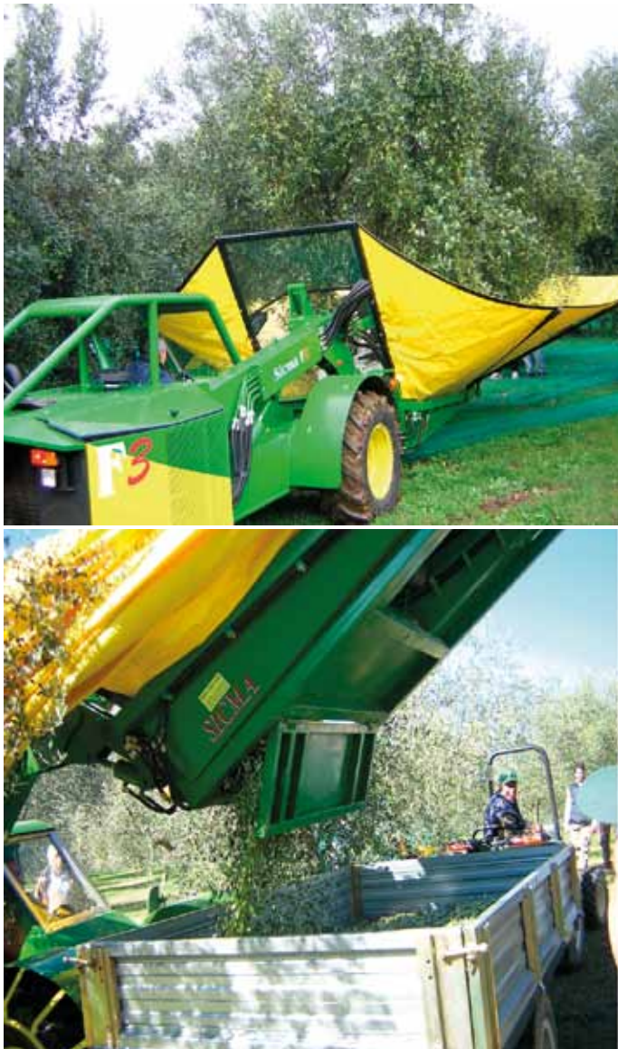
Fig. 1 - Mechanical harvesting of olives with a trunk shaker with a reversed umbrella interceptor.
