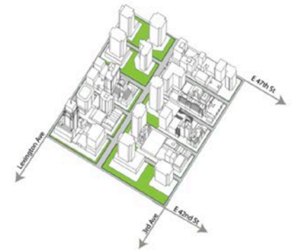
Green cover: 20% (33,769 m 2 ) — Street trees: 8,400 m 2 POPS: 25,369 m 2 Average change in air temperature: -0.58 OF
