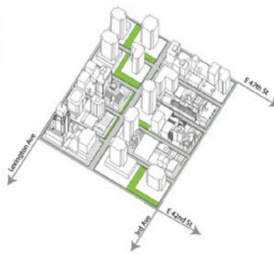
Green cover: 10% (16,885 m 2 ) — Street trees: 6,400 m 2 POPS: 10,485 m 2 Average change in air temperature: -0.45 OF
