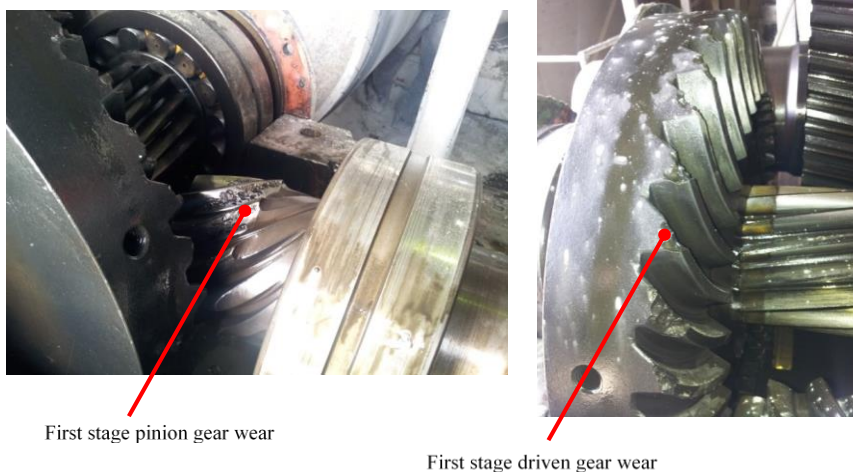
Fig. 17 Drive unit 4 – First stage gears wear
