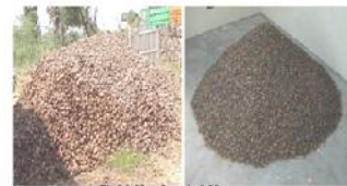
Fig.3.1. CS and crushed CS aggregate.
