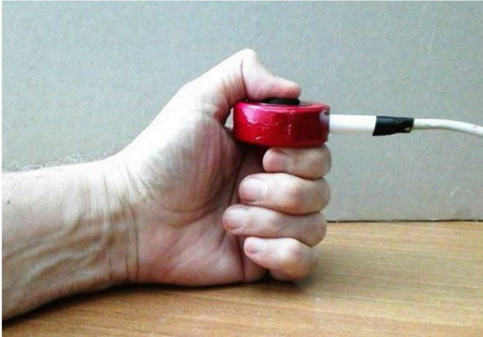
Figure 3 – Hand position for the measurement of pinch strength.
