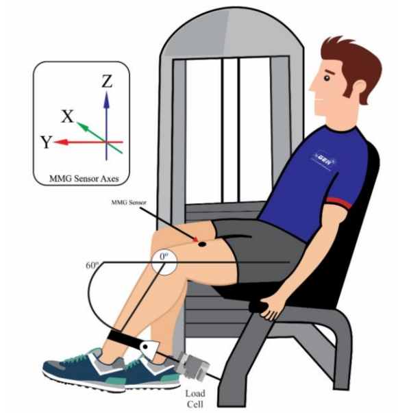
Fig. 1 Scheme of the experimental setup. The MMG sensor (triaxial accelerometer) was placed over the rectus femoris muscle belly and knee angle was positioned in 60^\circ of flexion with a load cell
