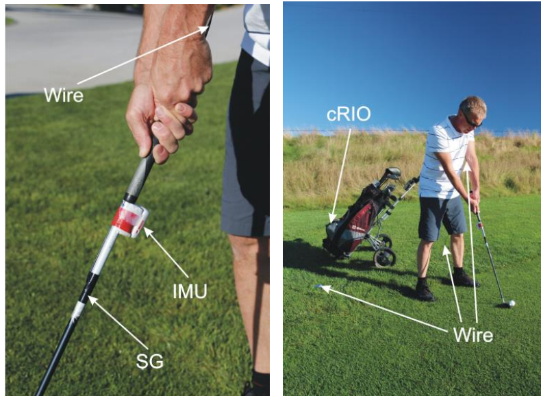
Fig. 3 Smart club prototype used in the field
