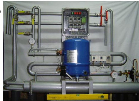
Fig. 2 Photo of the heat pump with coaxial evaporator and shell-tube condenser
