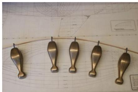
**Fig. 1** Example of drawing a spline with lattice
