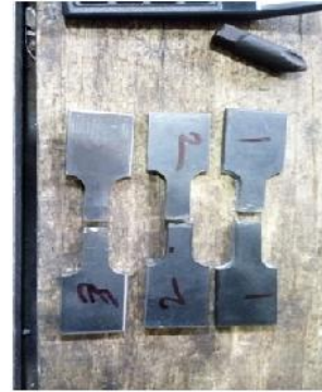
Fig.4.3. Dumbbell shape work pieces for tensile test.
