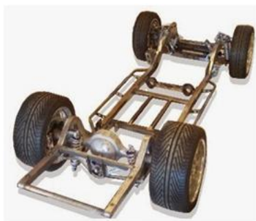
Fig.2.1. Conventional chassis or frame-full chassis.
