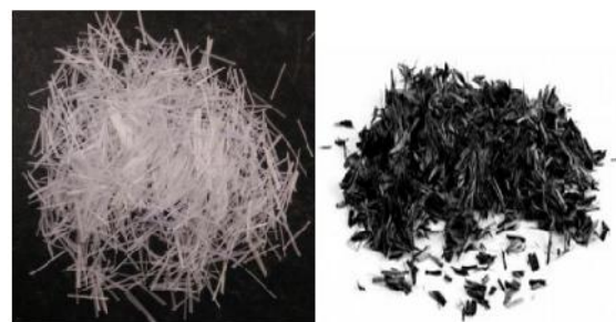
Fig.4.1. glass fiber and carbon fiber used for fiber reinforced concrete.
