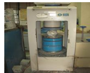
Testing of High Strength SCC cylinder of M100 grade for Split tensile strength
