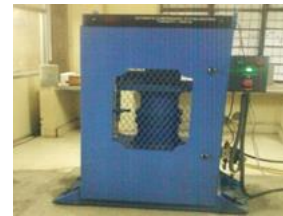
Testing of High Strength SCC cube of M100 grade in compression testing machine
