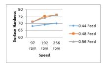
Surface Hardness Vs Speed by keeping force, number of passes constant of 98% aluminium+2% zirconium
