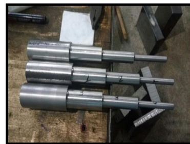
Fig: 2 – Machined EN 8 material during Turning Process
