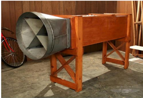
Fig 4. Wright Brothers 1901 Wind Tunnel [Source: Wright Brothers Aero plane Co. 2017. THE 1901 WRIGHT WIND TUNNEL . [ONLINE] Available at: http://www.wright-brothers.org/Adventure_Wing/Hangar/1901_Wind_Tunnel/1901_Wind_Tunnel.htm ]
