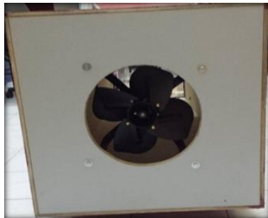
Fig 10. Exhaust fan kept in diffuser
