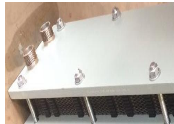
Figure 5.1 shows inlet and outlet with fins and the fastening ability to make it as compact as possible to fulfil the required position for test setup as required
