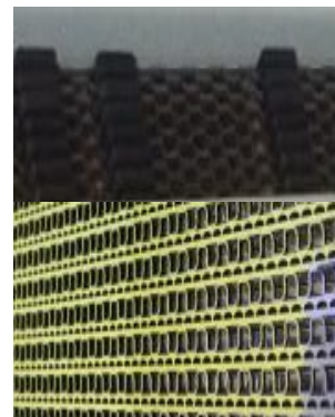
Figure 5.2 shows fins arrangement and beading arrangement with fins of cross flows wave type without disturbing the flow .
