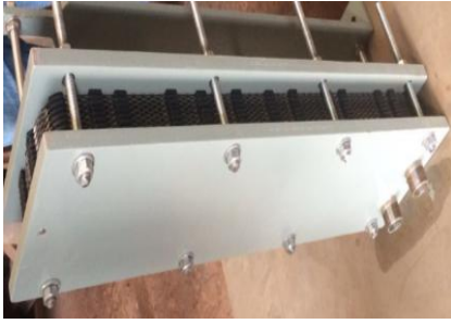
Figure 5.3 shows the compact heat exchanger final fabrication assembly and the area enhancement for further application research of performance testing analysis with different fluids, flow rates and different pressures.
