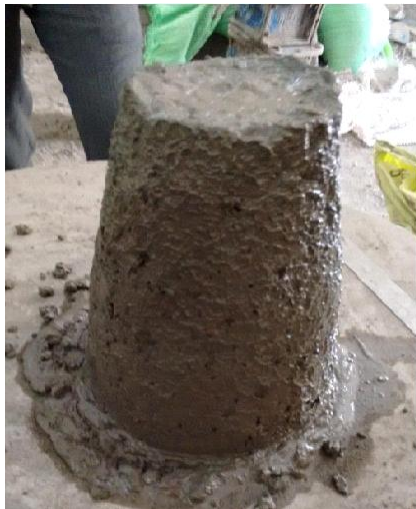
Slump Test Conducted
