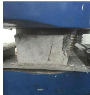
After applying compressive strength on cube
