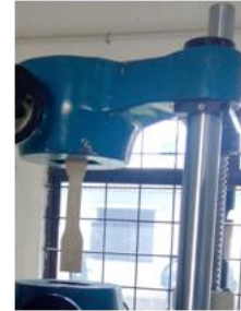
Fig. 1. Tensile Test Specimen loaded in UTM
