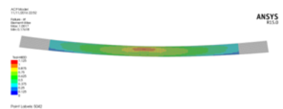
Fig. 10. IRF plot for Eglass/Epoxy under Load set2 (excluding edges)
