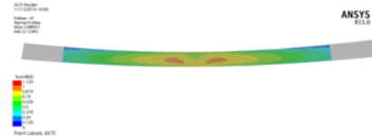
Fig. 14. IRF plot for HC2 under Load set2 (excluding edges)
