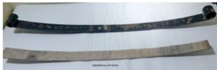
Fig. 3. EGLASS/EPOXY LEAF SPRING
