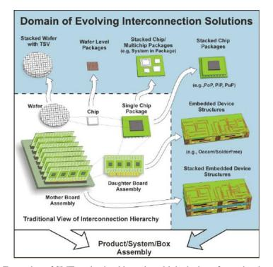
Fig. 5-7 Expansion of SMT packaging hierarchy with inclusion of new developments in packaging, including wafer levels and 3D stacks.
