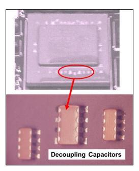
Fig. 4-1 Flip-chip column grid array (CGA) with exposed decoupling capacitors.
