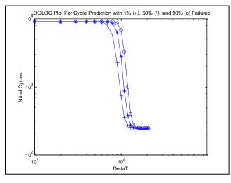
Fig. 7-12 Log-Log plot of projected cycles-to-failures versus temperature cycle range
