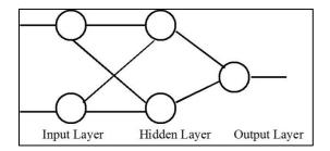
Fig. 7-2 Schematic of a simple ANN structure with a one hidden layer
