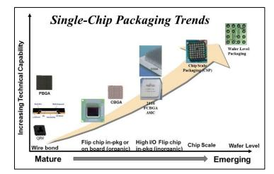
**Fig. 2-2** Single-chip packaging trends from ball grid array (BGA) to wafer level packages (Fan-in or Fan-out).
