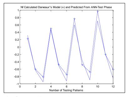
Fig. 7-5 Cycles-to-failure (+) and prediction using ANN CEP algorithm
