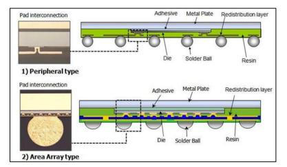
**Fig. 4-4** A new embedded package, wide strip fan-out package (WFOP), which uses a metal plate like.
