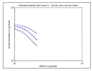
Fig. 7-11 Predictions of cycles-to-failures at 10% (o), 50%(\*), and 90% (+).
