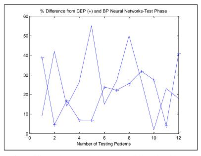
**Fig. 7-6** The difference between calculated and prediction using either CEP (+) or Backpropagation ANNs
