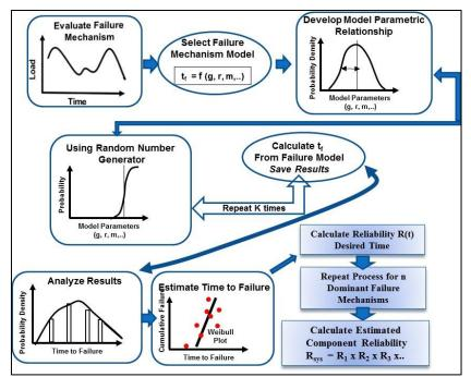
Fig. 6-3 Virtual qualification process by Monte Carlo simulation
