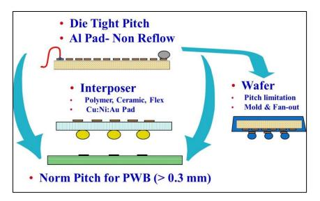
Fig. 2-1 Single-chip packaging concept from wire-bond to flip-chip ball grid array to wafer-level packaging (fan-in and fan-out).
