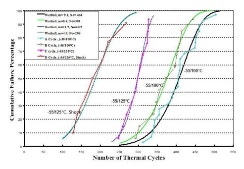
Fig. 7-7 Cycles-to-failure for CBGA 625 assemblies under different cycling conditions
