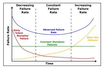
Fig. 6.2 Classic bathtub reliability curve showing the three stages during the life of a product from a reliability perspective: infant mortality, steady-state, and wear-out.
