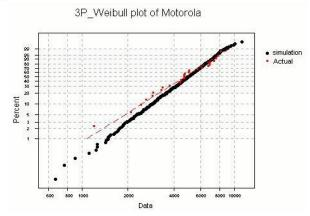
**Fig. 6-4** 3-P Weibull plots of simulation and actual test data for the 0/100C thermal cycle condition.
