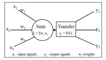
Fig. 7-1 Schematic of an ANN structure
