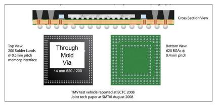
Fig 3-3 Cross-section top and bottom view of a new TMV<sup>™</sup> PoP package [19].
