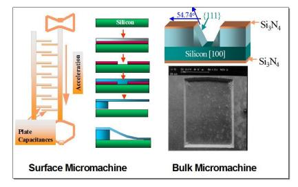
Fig. 5-1 Surface and bulk micromachining fabrication and structure
