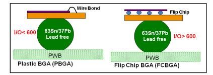
**Fig. 2-3** Typical plastic ball grid array with internal wire-bond and flip-chip die for low and high-I/O package configurations, respectively.
