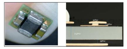
Fig. 4-5 Configuration of wafer level chip scale module package (WLCSMP).
