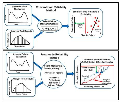
Fig. 6-5 Comparison of conventional reliability prediction methods to prognostic approaches that predict remaining useful life (RUL)
