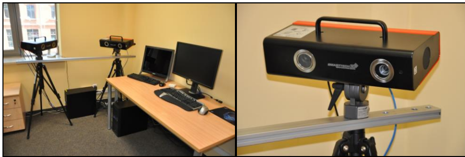
Fig. 5 MBS laboratory stand (left) and the structured light scanning device (right)
