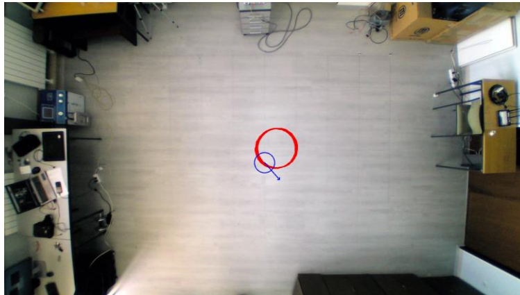
Fig. 2 Logged trajectory of circular motion of marker. Number of repetitive cycles is 30.
