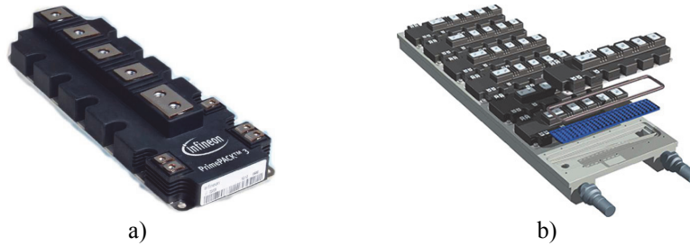
Fig. 3 a) a PrimePak™ 3 IGBT module, which is widely used in wind power applications [5]; b) CAD model of a power stack assembly for wind turbine inverters including fluid heat sink [6].
