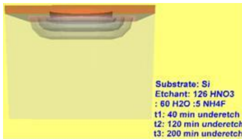
Fig. 6c Etching square mask (Marker String method) rendered , 2D view [84].
