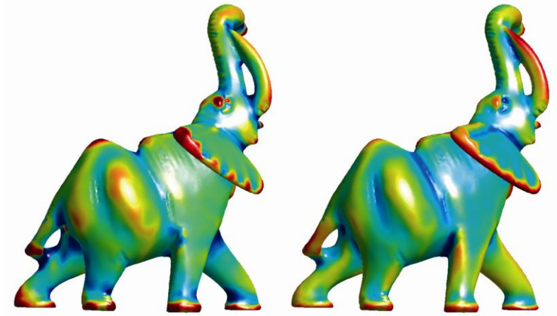
Fig. 3 The plot of Gaussian and mean curvature estimation respectively. Red colored areas are regions with a high level of curvature. The blue areas have low values of curvature.
