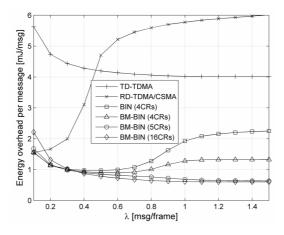
Fig. 10 Energy overhead per message of TDMA-based protocols under varying traffic load
