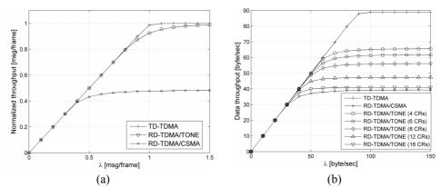
Fig. 9 Data throughput of TDMA-based protocols under varying traffic load: (a) normalized throughput and (b) data throughput
