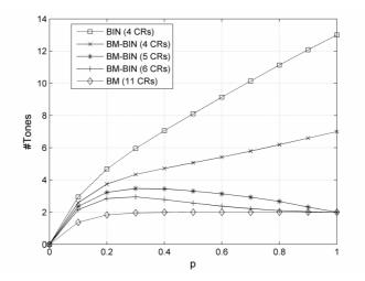
Fig. 7 The average number of generated tones per contention session in transmitter group of size 12 versus transmission probability for different group splitting algorithms
