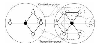
Fig. 3 Transmitter and contention groups in RD-TDMA/CSMA
