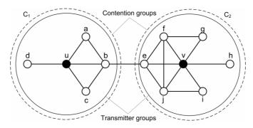
Fig. 6 Transmitter and contention groups in RD-TDMA/TONE
