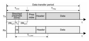
Fig. 2 Data transfer period of slot
