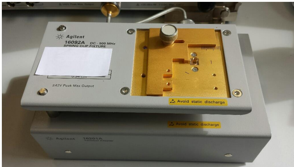
Fig. 10 Spring clip fixture and terminal adapter used for Pogo pin impedance – frequency measurement
