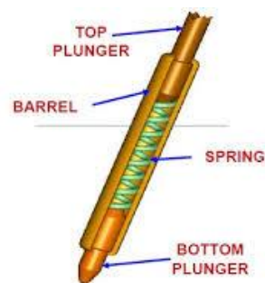
Fig. 8 Pogo pin internal structure
