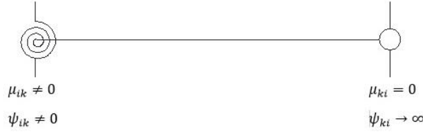
Fig. 5 Semi rigid connection at left node and connection with ideal hinge at right node
