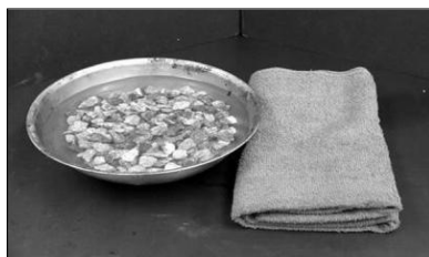
Fig.1. The soaking of coarse aggregates
