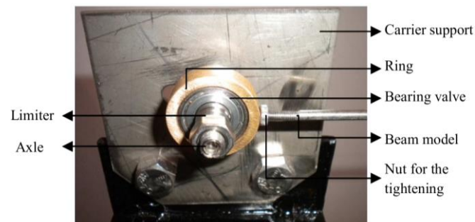
Fig. 5 Detail of pinned support
