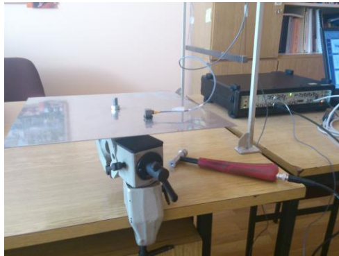
Fig. 12 Measurement equipment used for FRF testing
