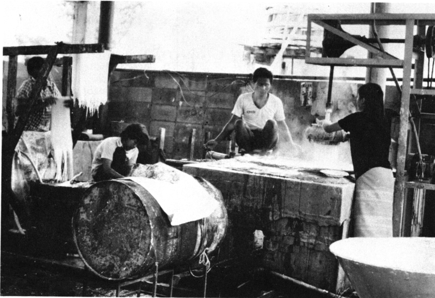
Extrusion and washing stages in a Thai noodle factory.
