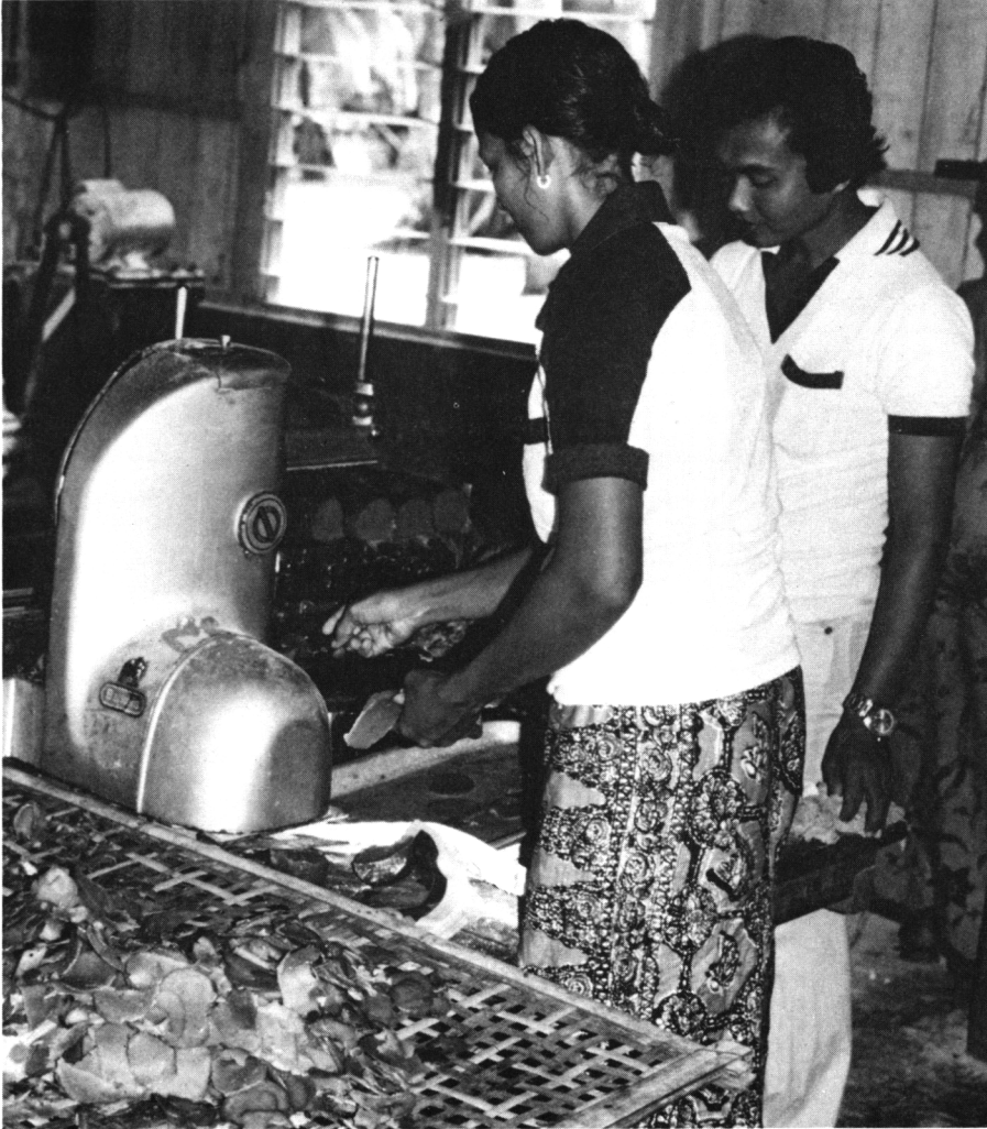
In small factories, some mechanical operations are important such as this dough-slicing operation in a fish cracker plant in Malaysia.
