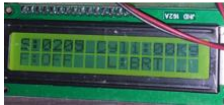
Fig4.1:LCD display shows the cylinder weight
