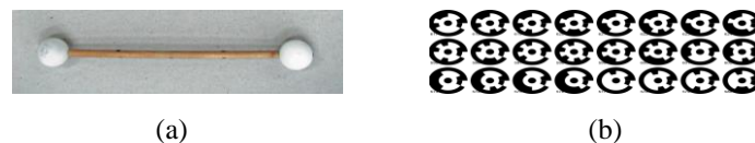
Fig. 2 (a) Experimental linear object: cylindrical wooden stick (l=25cm, diameter=10mm) (b) Printed “RAD” target panel (w=15cm, h=35cm) (Source: Djordjevic et al. [2])
