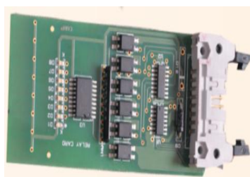
Figure 14: Relay Card – Prototype & Block diagram
