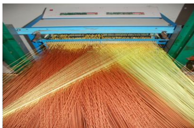
Figure 3: Hooks & Harness in Electronic Jacquard
