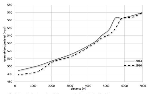
Fig. 7 Longitudinal section of the reservoir along the Radika River water course.
