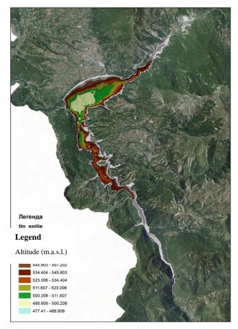
Fig. 2 Digital terrain model (DTM) of the Shpilje reservoir bottom
