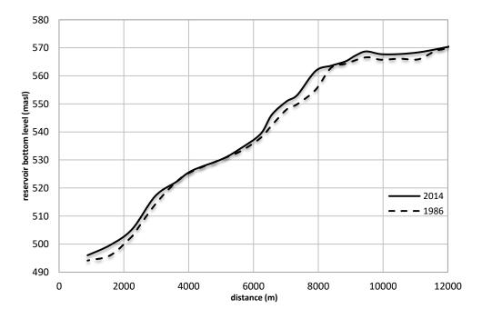
Fig. 6 Longitudinal section of the reservoir along the Crn Drim River water course
